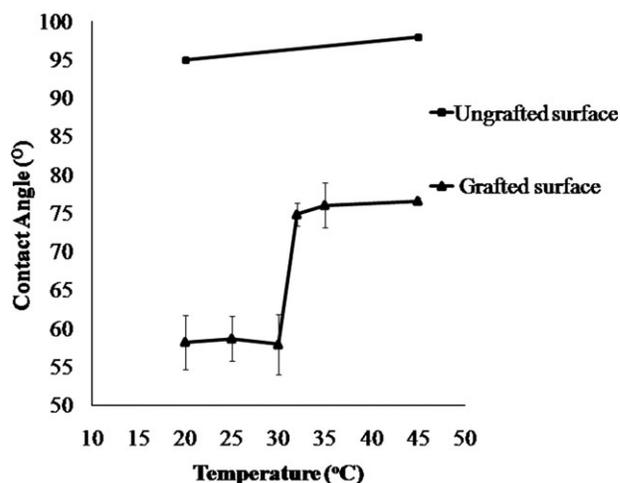
**Figure 2.** Contact angles of the PNIAm-co-AM grafted surface and ungrafted surface at various temperatures.
