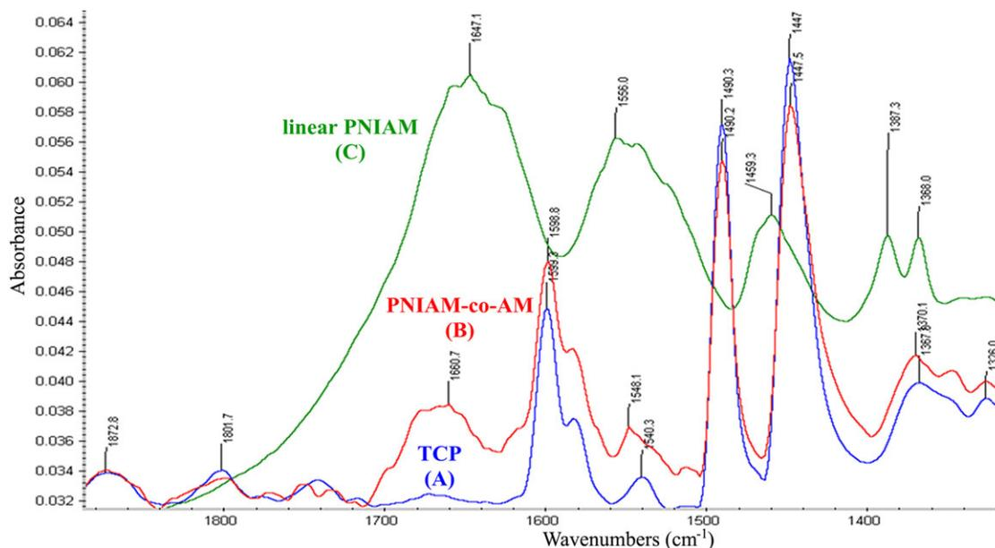
**Figure 1.** FTIR spectra of (A) ungrafted TCPS, (B) PNIAm-co-AM grafted TCP surface and (C) linear PNIAm, for wavenumbers ranging from 1800 to 1400  $\text{cm}^{-1}$ . The peak at around 1660  $\text{cm}^{-1}$  represents the secondary amide in the AM copolymer. [Color figure can be viewed in the online issue, which is available at [wileyonlinelibrary.com](http://wileyonlinelibrary.com).]
